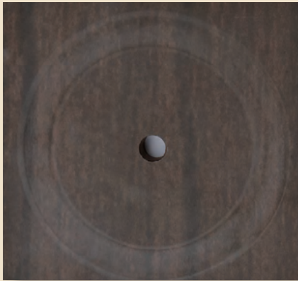
南亞舒活地板 (10,000轉) : 僅少許磨耗 Nan Ya Eco flooring tile (10,000 turns) : Only a little surface has been grinded
